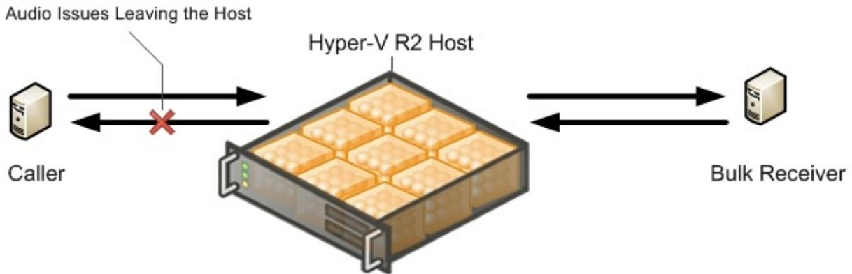
The following image indicates that the sent (transmit) "leg" is usually the first to have quality problems. This problem is a result of the variability of the data transfer of recordings with RTP streams from Interaction Media Server to another network storage location. The receive (sent) "leg" only has RTP streams coming into Interaction Media Server, but the problem will occur after a longer period of time. For this reason, it is important to evaluate both sides of the RTP steaming channels.
