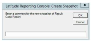
3. In the box, type a name for the snapshot and then click **OK**. The system saves the snapshot under the original report node in the **Navigation** pane.
