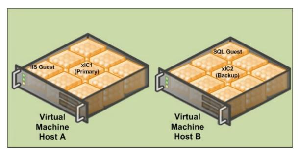
If Power is lost to Host A, the VM software detects the failure and tries to restore the servers running on Host A.In the meantime, the server on Host B has taken over the call processing. The state information is lost just as it would be with a real server.
