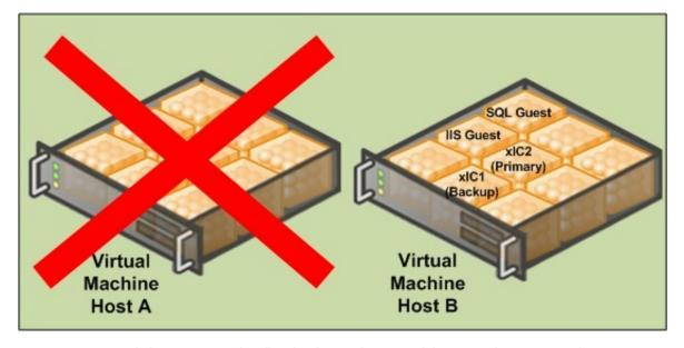
It is not recommended to move VMs handling load in production. In lab testing, the timing can be sensitive on machines handling multiple interactions per second. Some real-time data can be potentially lost. It is for this reason that-in a VMware environment - we strongly recommend assigning VMotion traffic to a dedicated NIC.Live Migration traffic should also run on a separate NIC away from the guests and management traffic.
