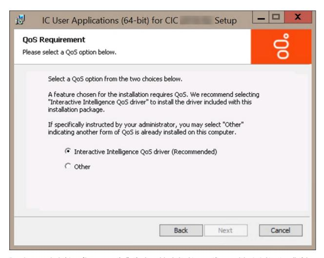
**PureConnect QoS driver (Recommended):** If selected, both the driver certificate and the QoS driver install. If the current permissions on the workstation do not allow modification of the Trusted Publishers list, a message indicating such appears.
