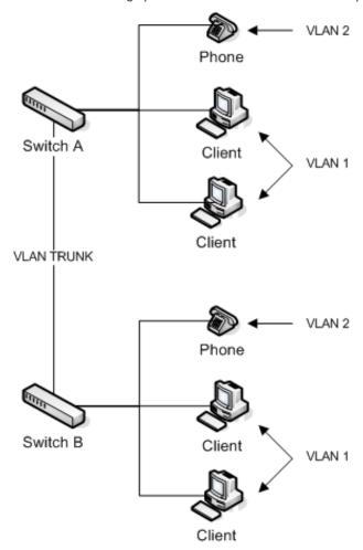
Set up the VLAN trunks on both of the switches. Run these commands on both switches.
