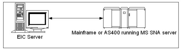
Another possible configuration which may improve performance over the first implementation is to run the SNA and CIC server on the same machine. In this configuration, the CIC server can access the SNA exposed API to retrieve data directly from the mainframe. The problem with this configuration is that you have to run non-CIC processes on the CIC server, reducing its reliability. This implementation is shown in the following figure:
