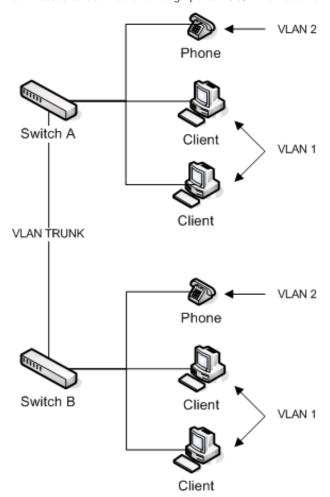
1. Set up the VLAN trunks on both of the switches. These commands must be run on both switches. From the privileged exec mode:
