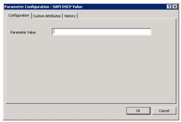
5. In the **Parameter Value** box, type 0x0 and then click **OK**. The new server parameter and its value appear at the bottom of the table in the right pane of the **Interaction Administrator** window.
