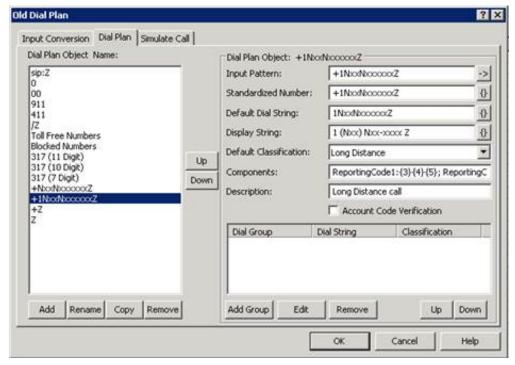
The Dial Plan processing starts after the input conversion step has created a standard Output Pattern of the phone number input. If the conversion step did not match the input with a predefined input pattern, the dialed number is passed directly (unformatted) to the Dial Plan table for processing. In either case, Dial Plan attempts to match the standardized or unformatted input it receives with its own input pattern list to take the appropriate dialing action.
