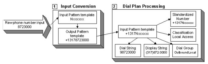
The first-generation dial plan comes with two basic phone number pattern tables: **Input Conversion**, which maps user input into standard phone number formats, and **Dial Plan**, which uses a predefined dial object. Dial Plan determines how to dial the number, what to display for the user, what the dialing permissions are and which outbound line to use to dial the number.
