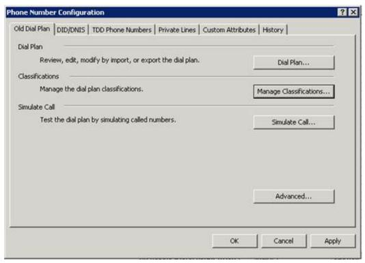
Select the **Dial Plan** button to display the **Input Conversion** and **Dial Plan** configuration tabs. The **Simulate Call** tab on that page is the same as the page launched by the **Simulate Call** button.
