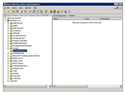
3. In the new OU, add the workstations that you wish to receive the software installation, in this case, the IC User Applications installation.
