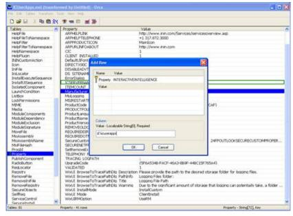
8. Close the **Add Row** dialog and click the **Features** table in the **Tables** column. Whether or not a feature is installed is determined by the value found in the **Level** column in the **Features** table. A value of **0** means a feature is disabled; a value of **1** means the feature is installed and a value of **100** means a feature is not installed.
