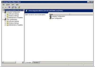
8. Select Computer Configuration...Software Settings...Software installation.
