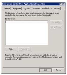
4. Click the Add button to add the transform to the IC User Applications installation package.
