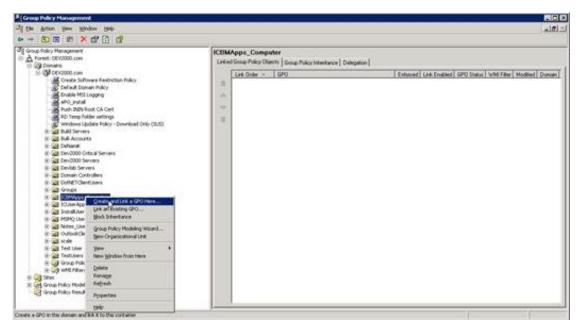
5. Give the GPO a name. In this example, the GPO is named ICBMAppsInstall.
