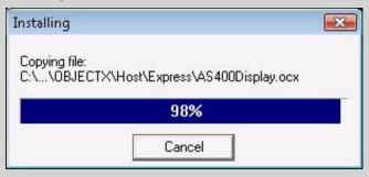
Instruct users to allow the installation to continue. They should *not* click the **Cancel** button - doing so may corrupt the installation or cause it to fail.
