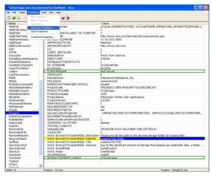
11. Orca will generate the transform and prompt for the transform filename (.mst) and location where it will be saved. In this example, the transform filename is MyTransform.mst and it is saved in the \ICUserAppsInstall directory on the local machine.
