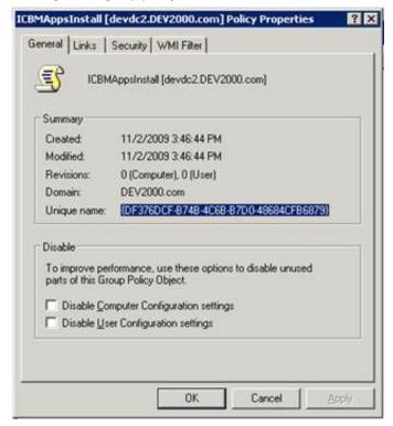
9. In Windows Explorer, locate the folder with the Unique Name value under the Windows\SYSVOL\domain\Policies folder. Place the script in the Machine\Scripts\Startup folder there. In this example the script is named ICBMApps\_InstallScript.vbs. Windows Explorer can be closed after placing the script.
