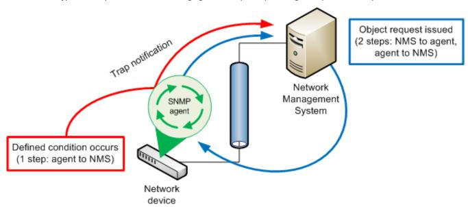
SNMP requests are issued from a Network Management System (NMS) to an SNMP agent service on a host network device. The request can be a query for status of a particular object, as defined in a Management Information Base (MIB) file, of the host network device. A request can also be a command to set a variable, such as a specific value for an object defined in a MIB file. When the request is received, the SNMP agent responds with a message to the NMS that sent the request.
