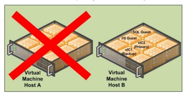
It is not recommended to move VMs handling load in production. In lab testing, the timing can be sensitive on machines handling multiple interactions per second. Some real-time data can be potentially lost. It is for this reason that-in a VMware environment - we strongly recommend assigning VMotion traffic to a dedicated NIC.Live Migration traffic should also run on a separate NIC away from the guests and management traffic.
