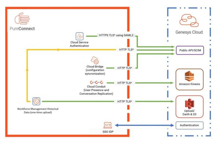
\*All traffic should operate using Transport Layer Security (TLS) v1.2 but can operate using TLSv1.0 for Amazon Kinesis and Amazon S3. For more information, see <u>Infrastructure security in Kinesis Data Streams</u> and <u>Infrastructure security in Amazon S3</u> in the Amazon Web Service Developer Guide.
