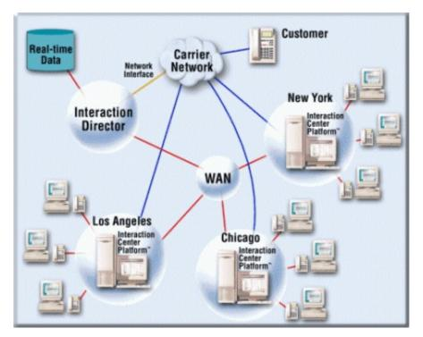
You can think of pre-call routing as "carrier-based routing" since routing decisions occur before the call connects and are based on signaling information from the carrier network.
