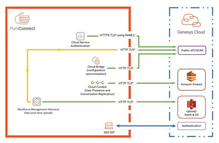
\*All traffic should operate using Transport Layer Security (TLS) v1.2 but can operate using TLSv1.0 for Amazon Kinesis and Amazon S3. For more information, see <a href="Infrastructure security in Kinesis Data Streams">Infrastructure security in Amazon S3</a> in the Amazon Web Service Developer Guide.
