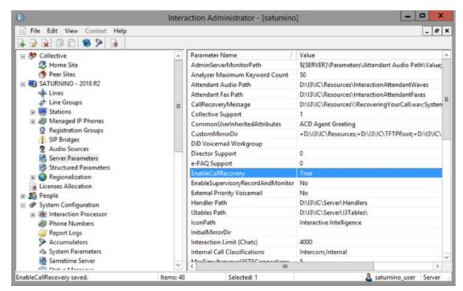
6. This server parameter is not dynamic; therefore, restart the TS server to imply a double switchover so that both the primary and the backup TS servers recognize the new server parameter value.
