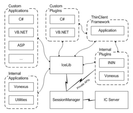
IceLib interfaces with SessionManager, the CIC subsystem that brokers connections between client applications and a given CIC server. Custom IceLib applications fully leverage SessionManager, just like internally developed CIC applications. For example, Interaction Desktop, Interaction Fax, and Interaction VoiceMail all use IceLib and take advantage of its SessionManager capability. IceLib is featurelicense based, not per-seat or per-session. Client sessions require client licenses, of course.
