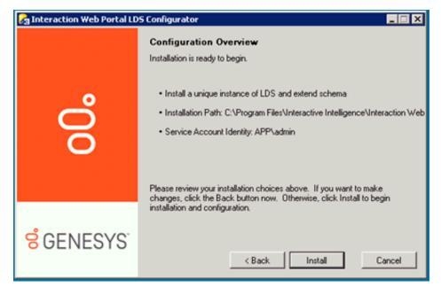
8. Click Install. The Configuration Progress dialog box appears and displays task installation progress check marks as the installation progresses.
