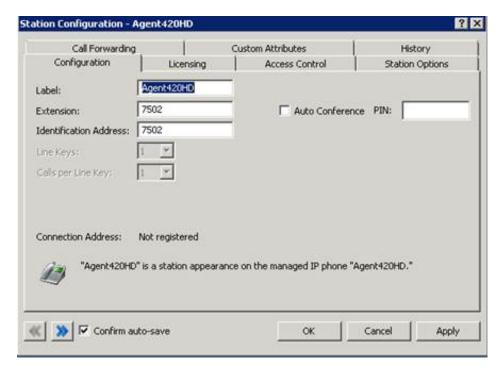
The SIP stations associated with managed IP phones are of the type Managed Workstation or Managed Stand-alone Phone.
