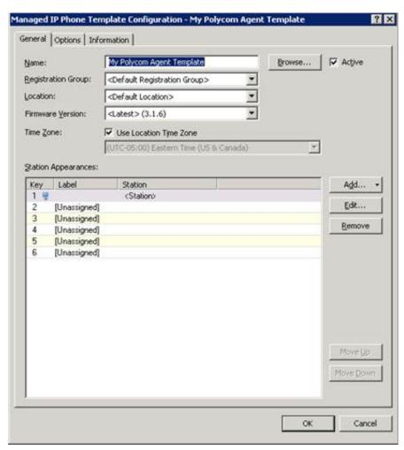
3. Select or add the appropriate configuration items in the **General** and **Options** (including **Advanced Options** for Polycom and Interaction SIP Station phones) tabs *for this managed IP phone template*.
