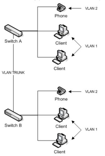
Set up the VLAN trunks on both of the switches. Run these commands on both switches. From the privileged exec mode:
