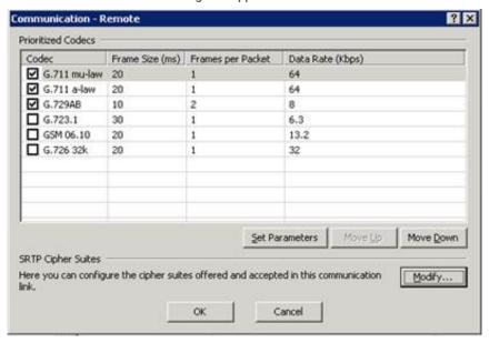
Since this server supports both LAN (high bit rate) connections and connects to the gateway and WAN, select both G.711 codecs. If you need to adjust any of the codec parameters, you can select **Set Parameters** to adjust the frame size and frames per packet, but this should rarely be necessary. If you need to modify the SRTP cipher suites, click **Modify**. Do not attempt to change the default settings, however, unless you are familiar with cipher suites concepts.
