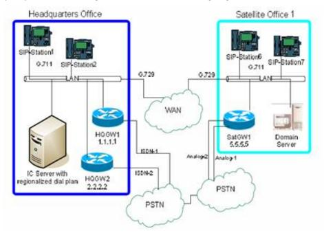
You can imagine additional satellite offices, each with a gateway connected to the PSTN, and one or more of these offices could be in different area codes, or some could support multiple area codes as local calls. On the Headquarters side, a separate SIP line on the CIC server would be dedicated to each gateway that services a satellite office. Such a configuration would require expertise to configure the gateway interface itself, which is not covered in this document.
