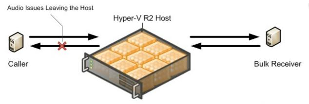
The following image indicates that the sent (transmit) "leg" is usually the first to have quality problems. This problem is a result of the variability of the data transfer of recordings with RTP streams from Interaction Media Server to another network storage location. The receive (sent) "leg" only has RTP steams coming into Interaction Media Server, but the problem will occur after a longer period of time. For this reason, it is important to evaluate both sides of the RTP steaming channels.
