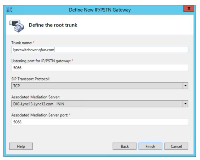
The Trunk name and Listening port fields auto-populate based on the FDQN specified on step 1. Specify the port on which the CIC server listens for requests, if different from the default port. The default port for TCP is 5066.
