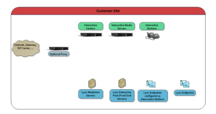
The following diagram shows the components for a PureConnect Cloud solution (local control model).
