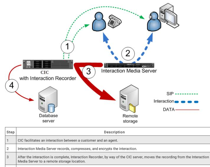
4 Interaction Recorder writes an entry to the database that identifies the recording and its location.
