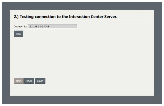
You must test the connectivity to the CIC server before the Next button will be enabled.
