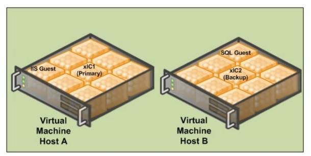
If Power is lost to Host A, the VM software detects the failure and tries to restore the servers running on Host A.In the meantime, the server on Host B has taken over the call processing. The state information is lost just as it would be with a real server.
